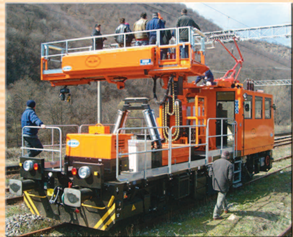
VMT 863 C with elevating and rotating platform
