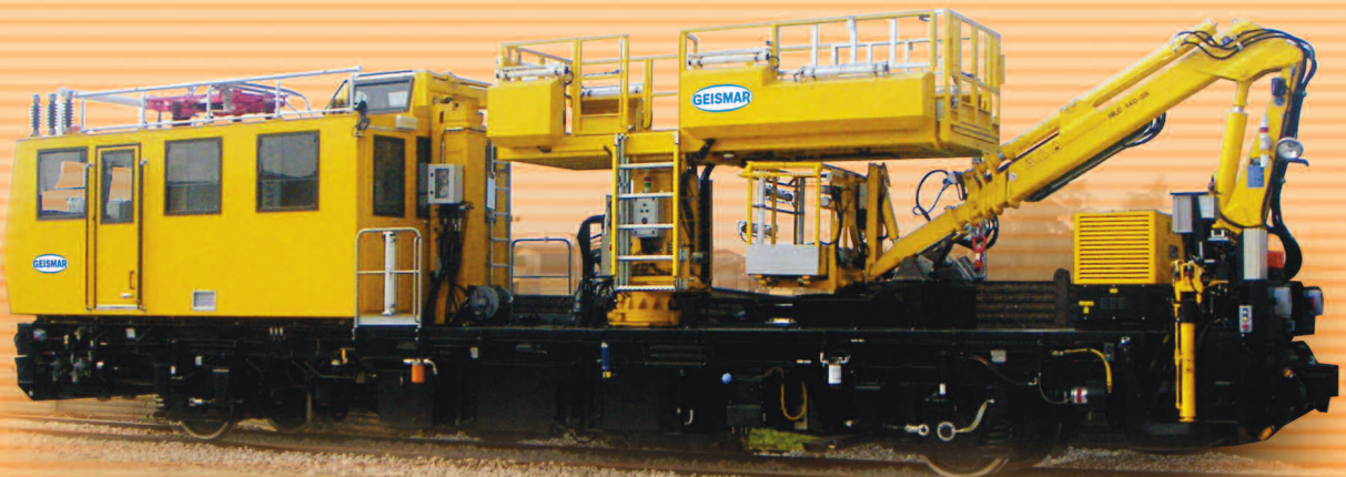
VMT 990 CGR heavy duty track motorcar with elevating platform and cradle elevator
